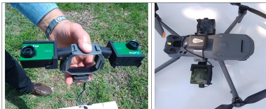
Figure 1. Used multispectral cameras mounted at DJI Mavic 3 UAV
