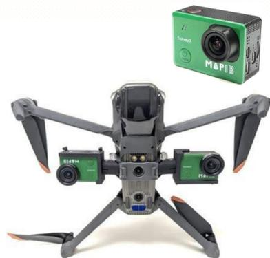
DJI drone with multispectral cameras MAPIR NGB and RGN - a view from below
